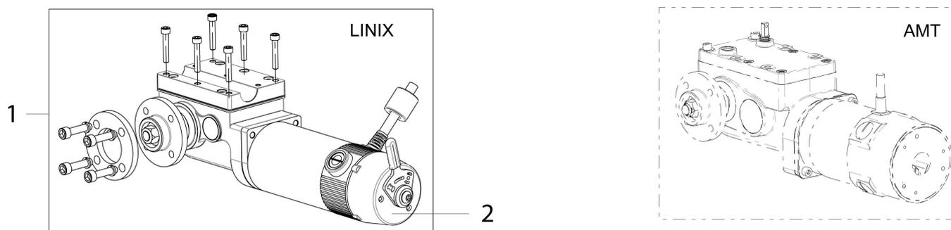
WITH MOTOR CHANGE ON GROOVE AMT MOTORS TO LINIX MOTORS THE CHAIR MUST BE REPROGRAMMED WITH JIVE M, JIVE F OR JIVE R FILE VIA WEB IQ
